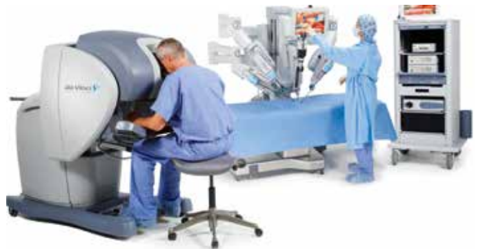
Figure 3 The da Vinci ® Robotic System, in which the surgeon operates seated at the console whilst the surgical team assists at the patient's side to change the robotic instruments
