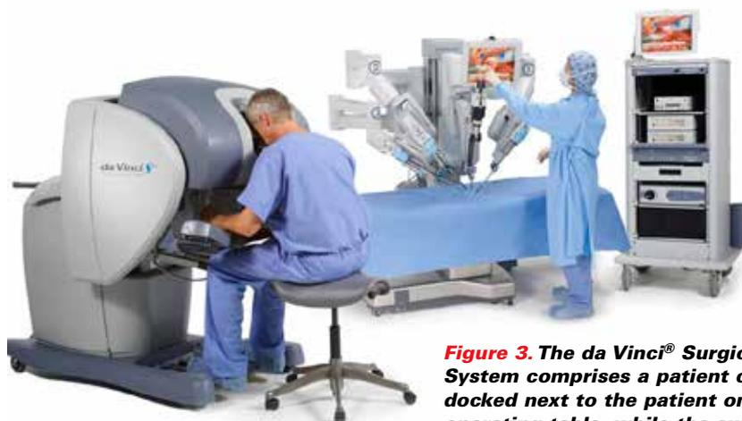
**Figure 3.** The da Vinci® Surgical System comprises a patient cart docked next to the patient on the operating table, while the surgeon operates from a console some distance away.
